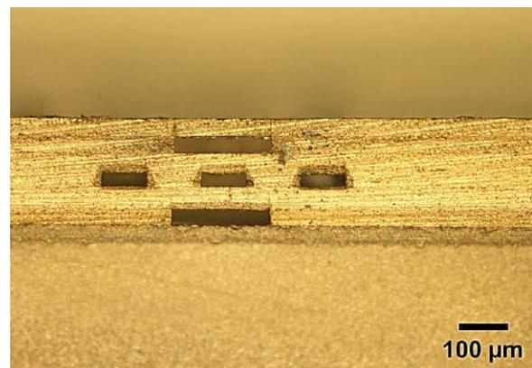
Fig. 1: Photo of cross-section of six laminated DFR layers. The total stack thickness was determined to be 213 μm.
