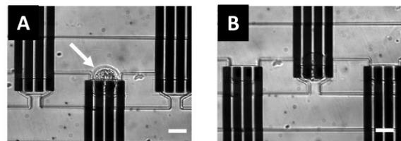
Fig. 2: Trapped oocytes. (A) With intact ZP, (B) without ZP. Scale bar: 50  $\mu\text{m}$ .
