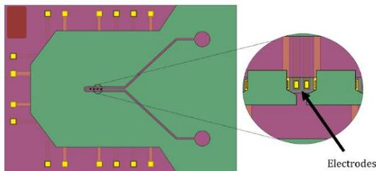
Fig. 1: Concept of microfluidic hydrodynamic traps with integrated microelectrodes for electrical impedance spectroscopy measurements.
