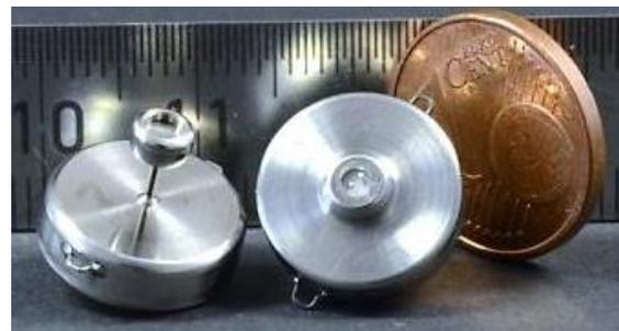
Fig. 8: Final design of a welded pressure sensor system for venous application
