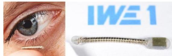
Fig. 2: Left: Proper dimensions of the sensor system; Right: Demonstrator of the glucose sensor system with silicone-molded ends
