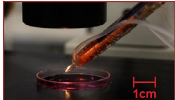
Fig. 1: Electromagnetic tweezers to move magnetical particles which were taken up by cells. The particles are hold by the cytoskeleton of the cells, moved by the tweezers and observed optically.
