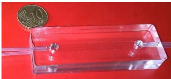
Fig. 4: Fluidic vessel made of PDMS to load adhered cells with shear stress due to flow of the liquid culture medium.
