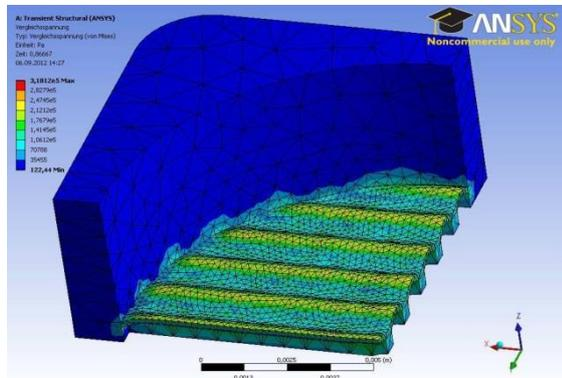
Fig. 3: FEM simulation of membrane bending due to pressure load.
