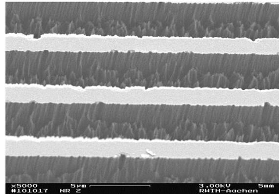
Fig. 5: Scanning electron microscope picture of a micro structured polyimide surface to investigate the influence of surface properties on cell development and growth.
