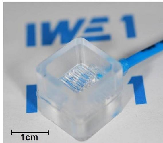
Fig. 2: Culture cavities made of PDMS with stretchable bottoms. Compressed air stretches the bottoms periodically. Adhered cells are also stretched.
