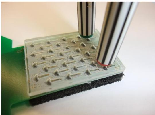
Fig. 1: Applying a load to a rigid tactile sensor array.
