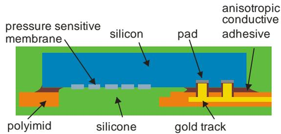
Fig. 3: Thin pressure sensor chip mounted on polyimide foil.
