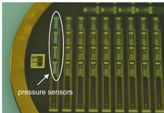
Fig. 4: Flip chip bonded pressure sensors before lapping
