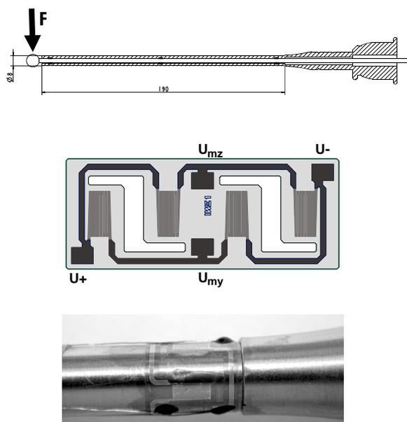
Fig. 3: Milling tool, sensor foil and sensor foil wrapped around the shaft of the milling tool
