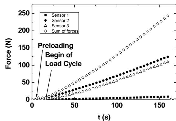
Fig. 2: Forces acting on one condyle in a compression test
