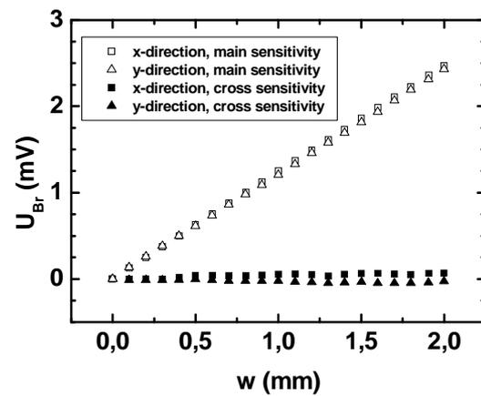
Fig. 4: Main sensitivity and cross sensitivity of strain gauge bridges in x and y direction
