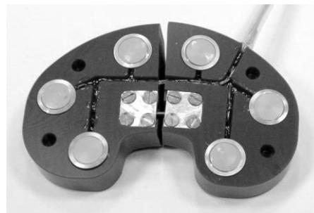
Fig. 1: Sensor-integrated tibial inlay
