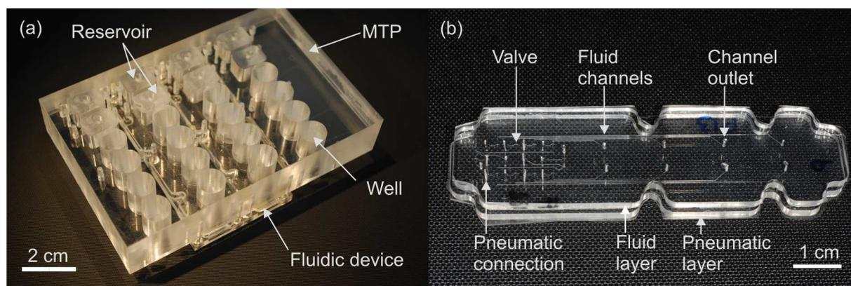
Fig. 1. (a) Microbioreactor made of PMMA with two microfluidic devices. (b) Microfluidic device made of PDMS
