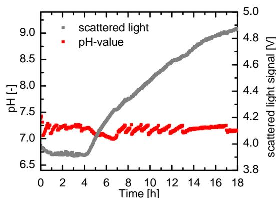
Fig.3. The pH-value und the scattered light signal of a pH controlled culture.
