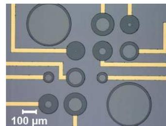
FIG. 1: Planar IrOx microelectrodes of different sizes
