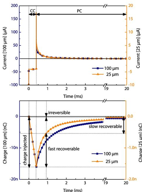
FIG. 3: Measured current of SIROF electrodes with different sizes and its correlated charge retrieved by integrating over time, after [9]
