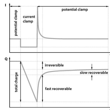
FIG. 2: Current and charge behaviour during pulse-clamp experiment
