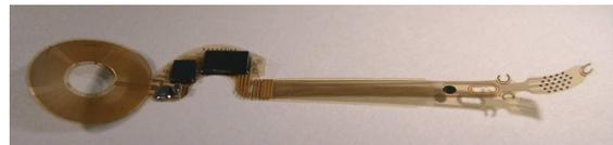
FIG. 2: Prototype of the EPI-RET-3 wireless retina implant
